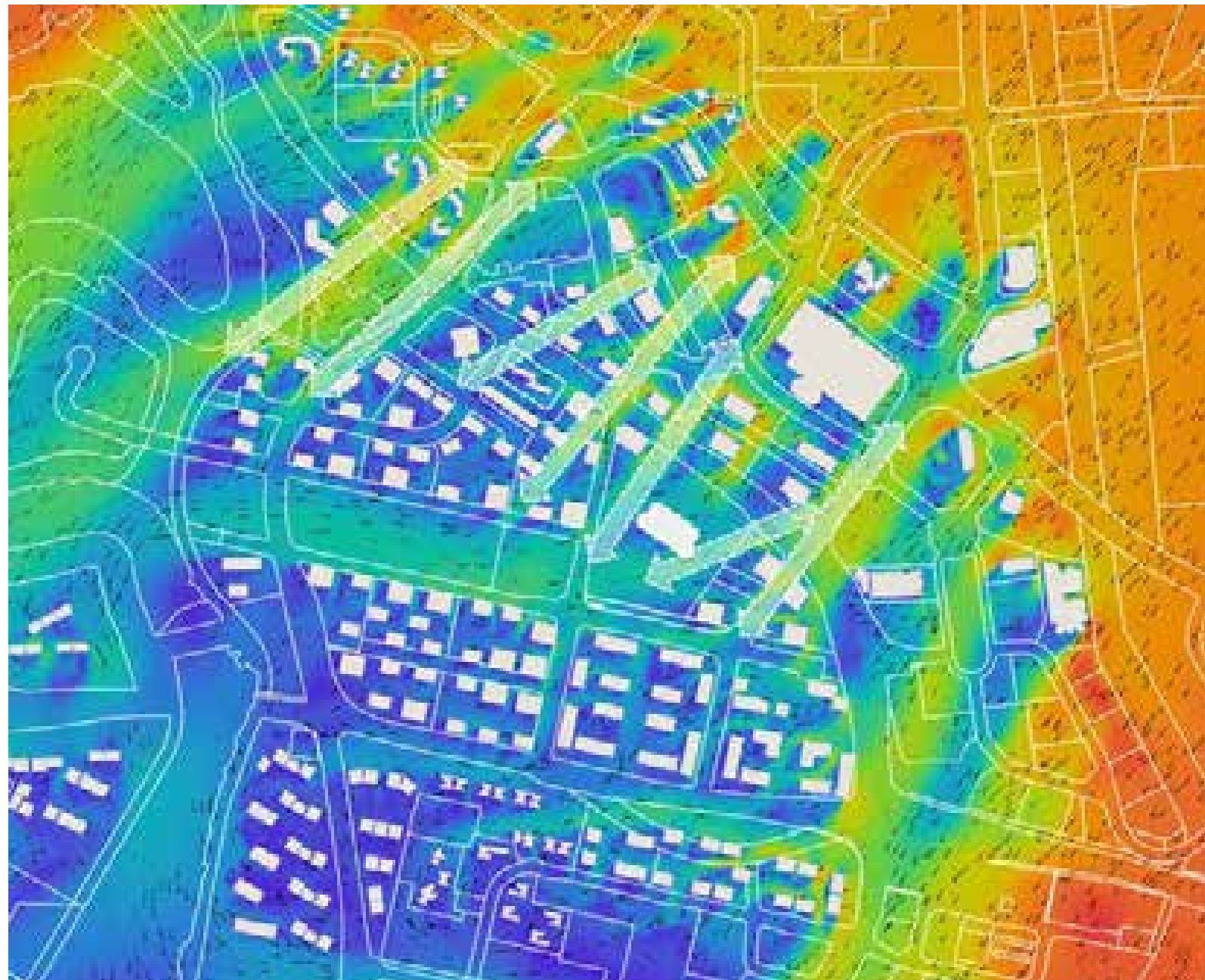
Wind flow environmental modelling of the precinct based on north-east wind Jurong Lake District Planning and Urban Design Guide
