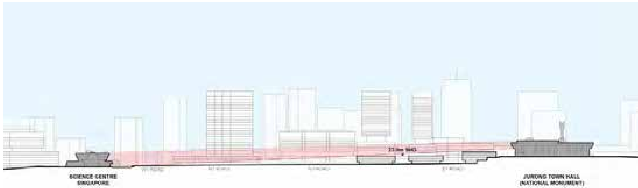
Conceptual section showing the view corridor that connects the Jurong Town Hall monument to the Science Centre Singapore main building
